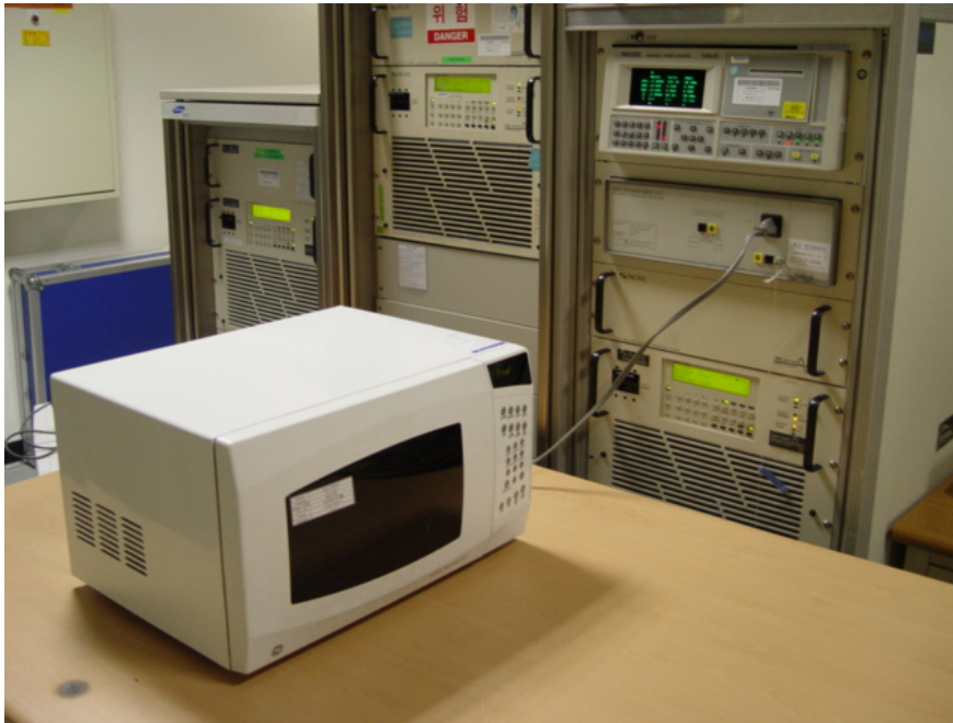
Fig.3 Test Setup for RF output power
