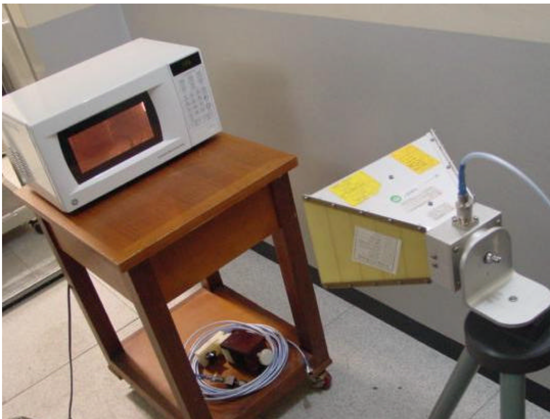
Fig. 5 Test Setup for Operating Frequency Measurements
