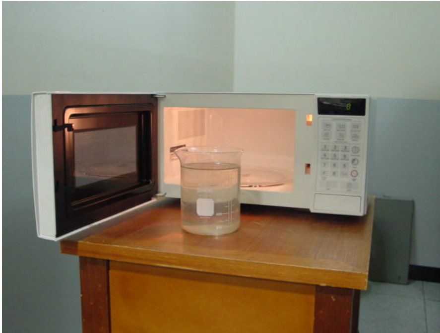
Fig.3 Test Setup for RF output power
