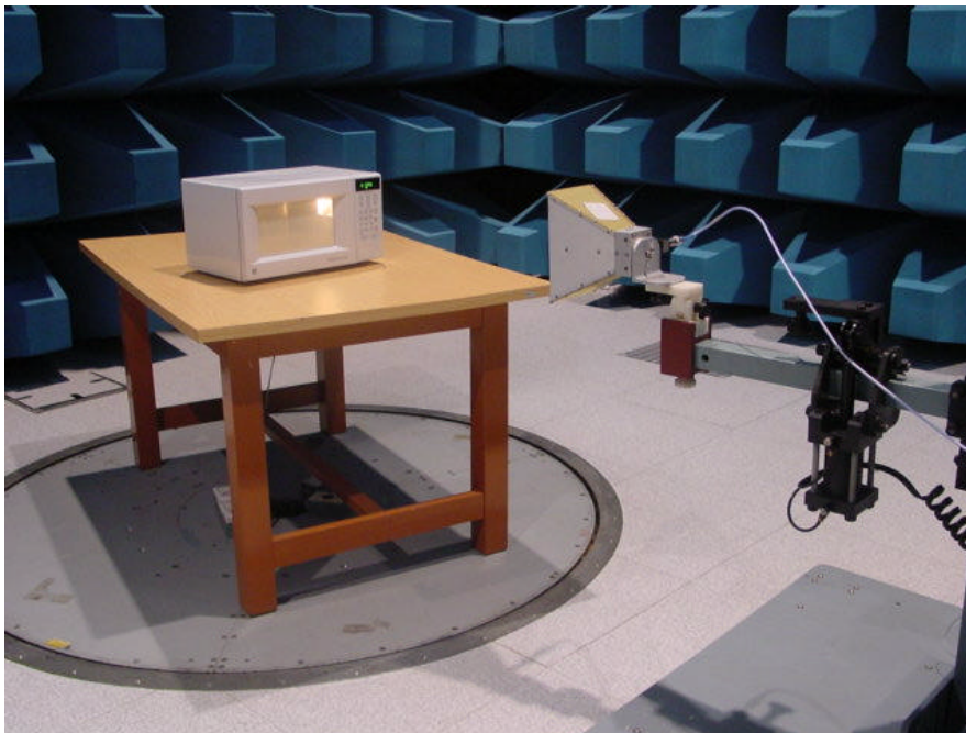
Fig. 9 Radiated Emission setup(1 - 25GHz)
