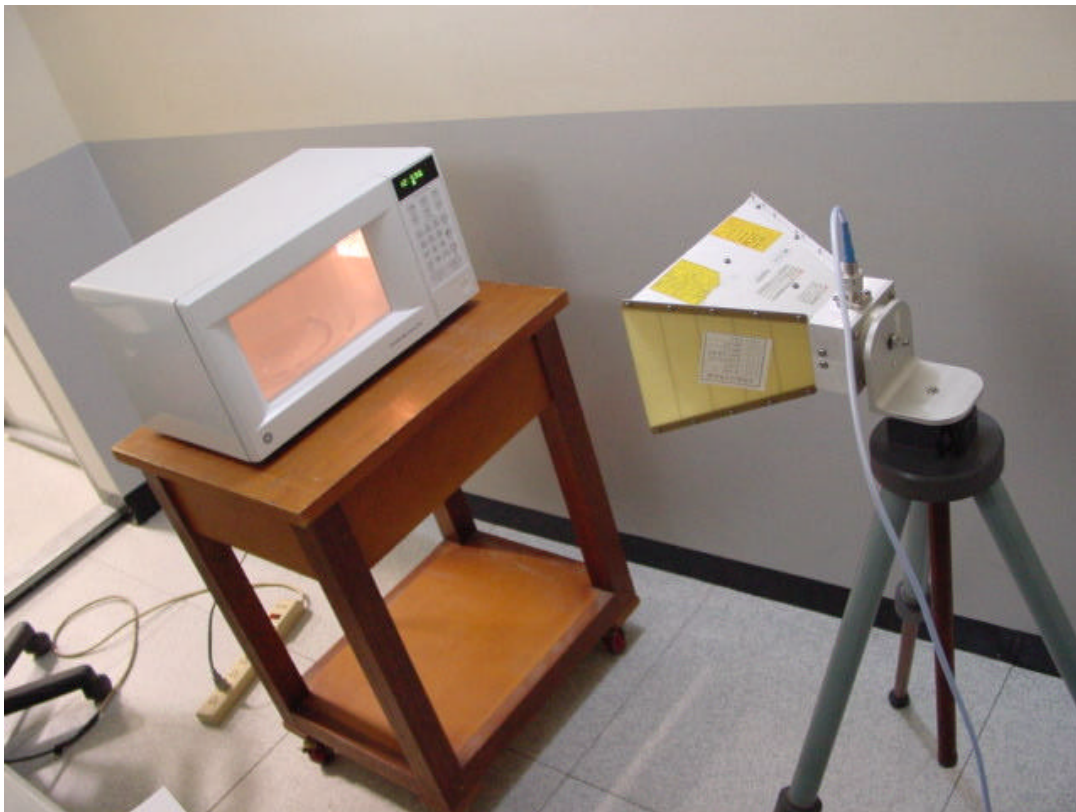
Fig. 5 Test Setup for Operating Frequency Measurements
