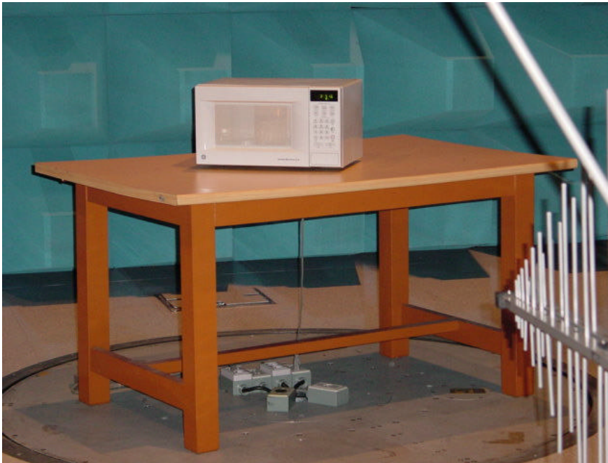
Fig. 8 Radiated Emission setup(30 - 1000MHz)
