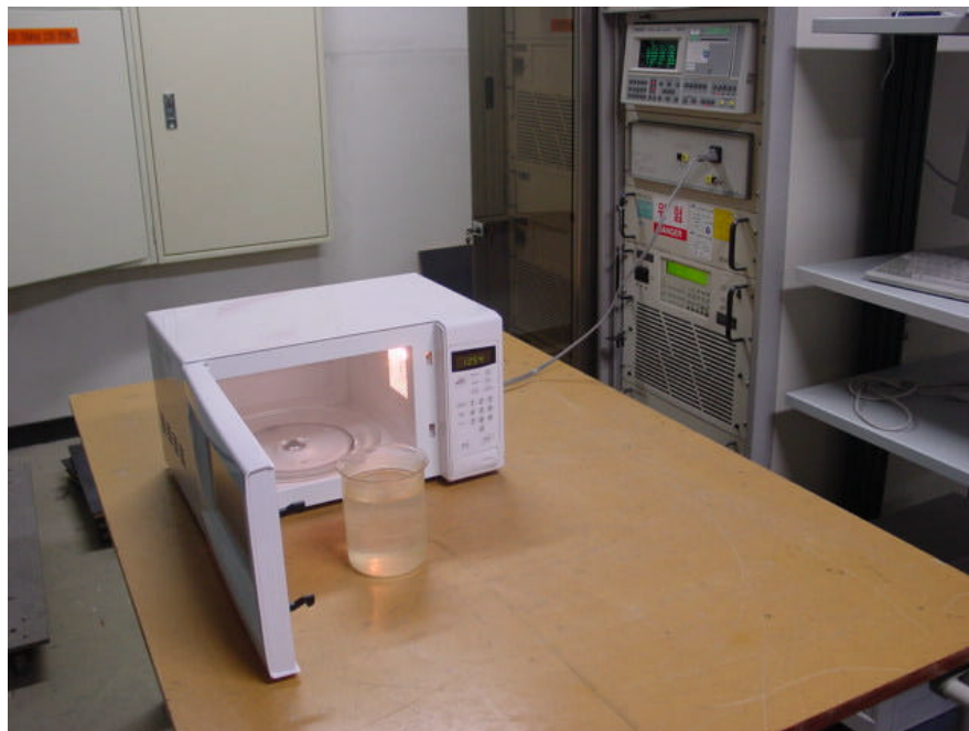
Fig.3 Test Setup for RF output power
