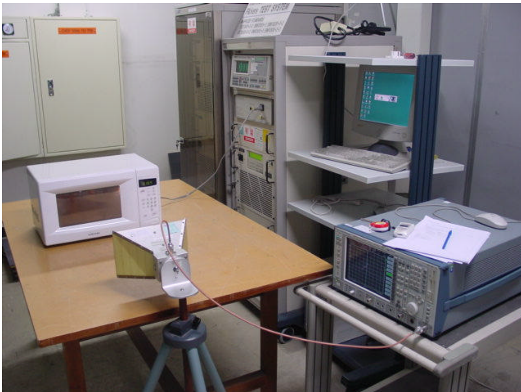
Fig. 5 Test Setup for Operating Frequency Measurements
