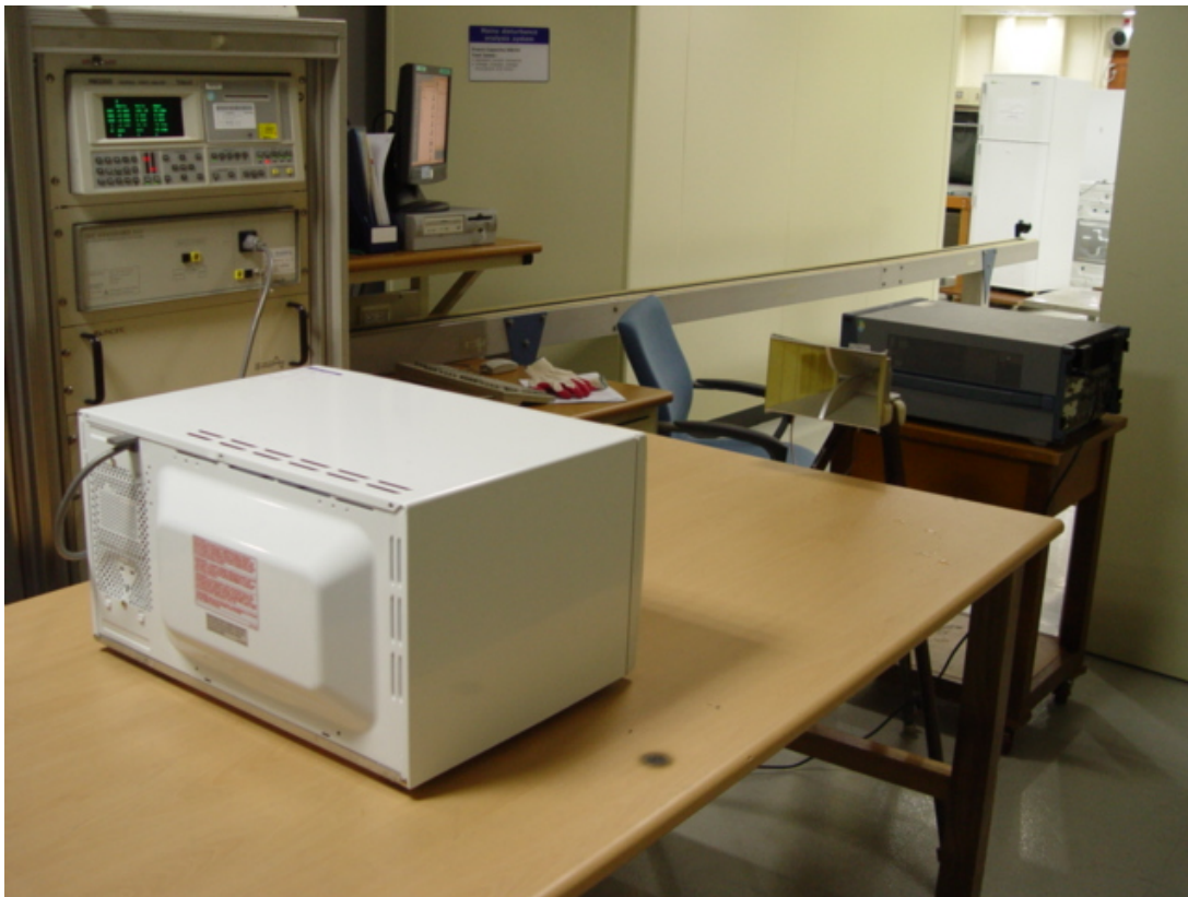
Fig. 4 Operating Frequency Measurements Configuration
