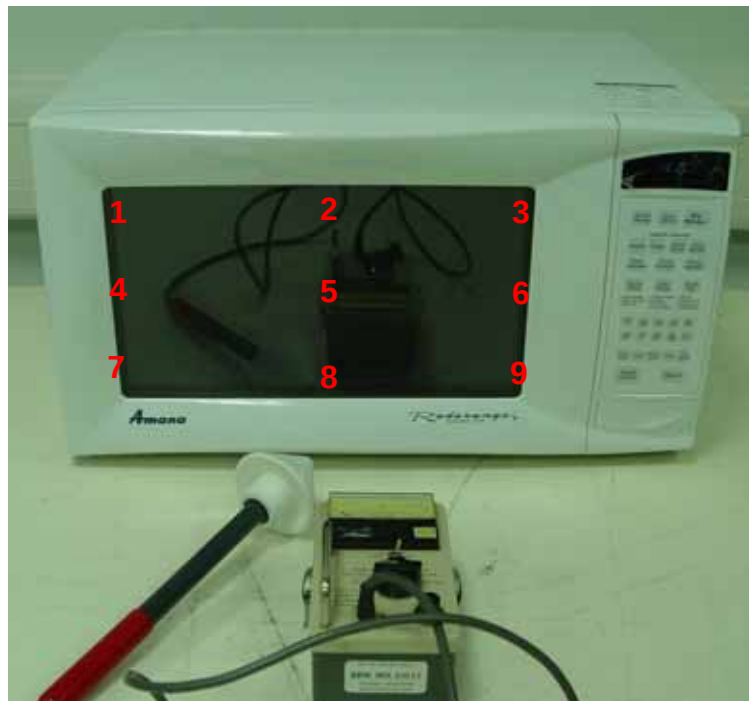
Fig. 1 Test Setup for Radiation Hazard Measurement
