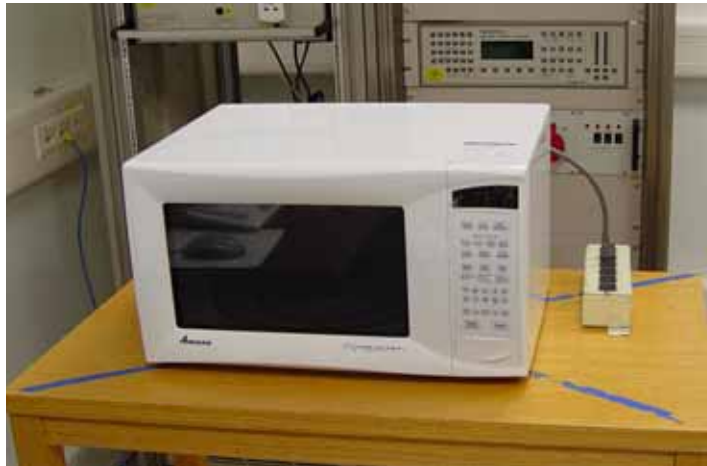
Fig.3 Test Setup for RF output power
