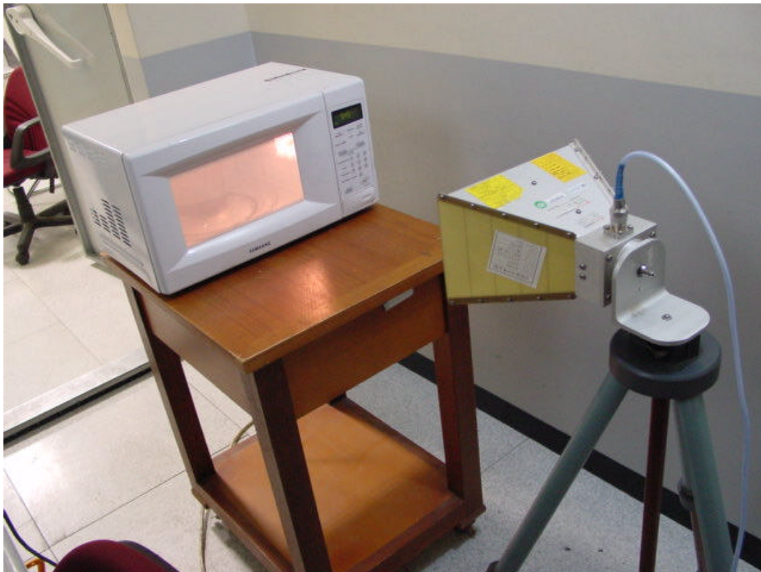
Fig. 5 Test Setup for Operating Frequency Measurements
