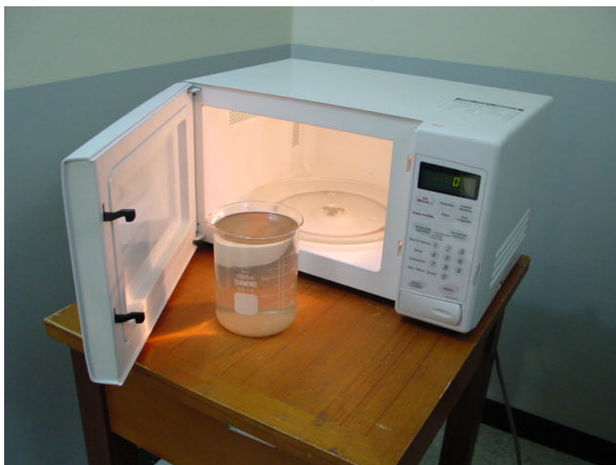
Fig.3 Test Setup for RF output power
