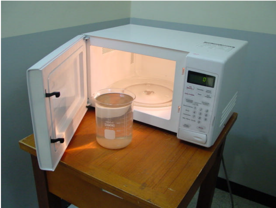
Fig.3 Test Setup for RF output power
