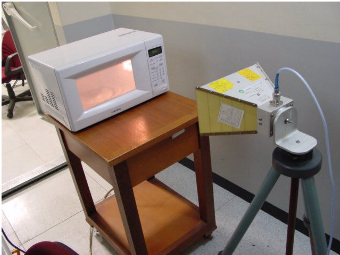
Fig. 5 Test Setup for Operating Frequency Measurements
