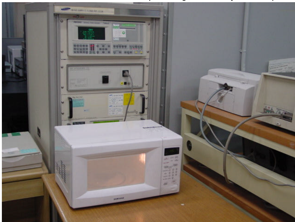
Fig. 2 Test Setup for Input power
