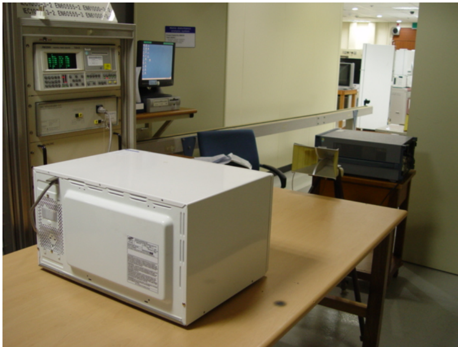
Fig. 2 Test Setup for Input power
