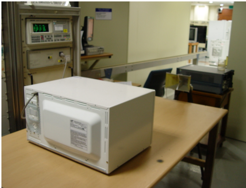
Fig. 2 Test Setup for Input power
