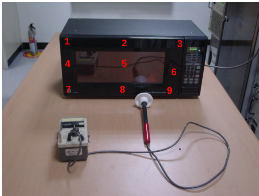
Fig. 1 Test Setup and the locations of maximum leakage
