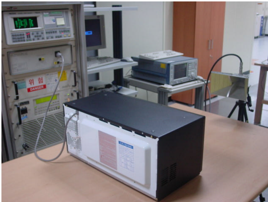
Fig. 2 Test Setup for Operating Frequency Measurements
