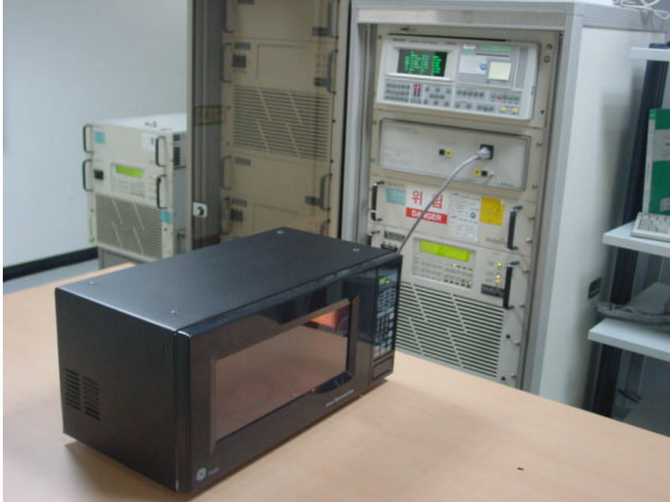
Fig. 2 Test Setup for Operating Frequency Measurements
