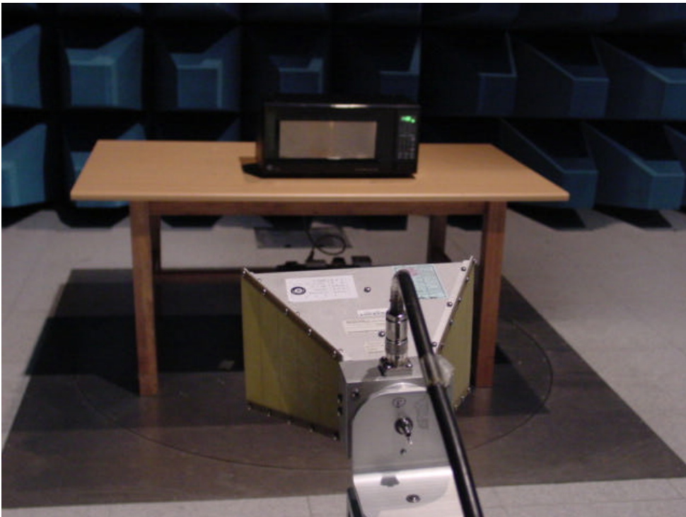
Fig. 4 Test Setup for Radiated Emission(1 - 25GHz)
