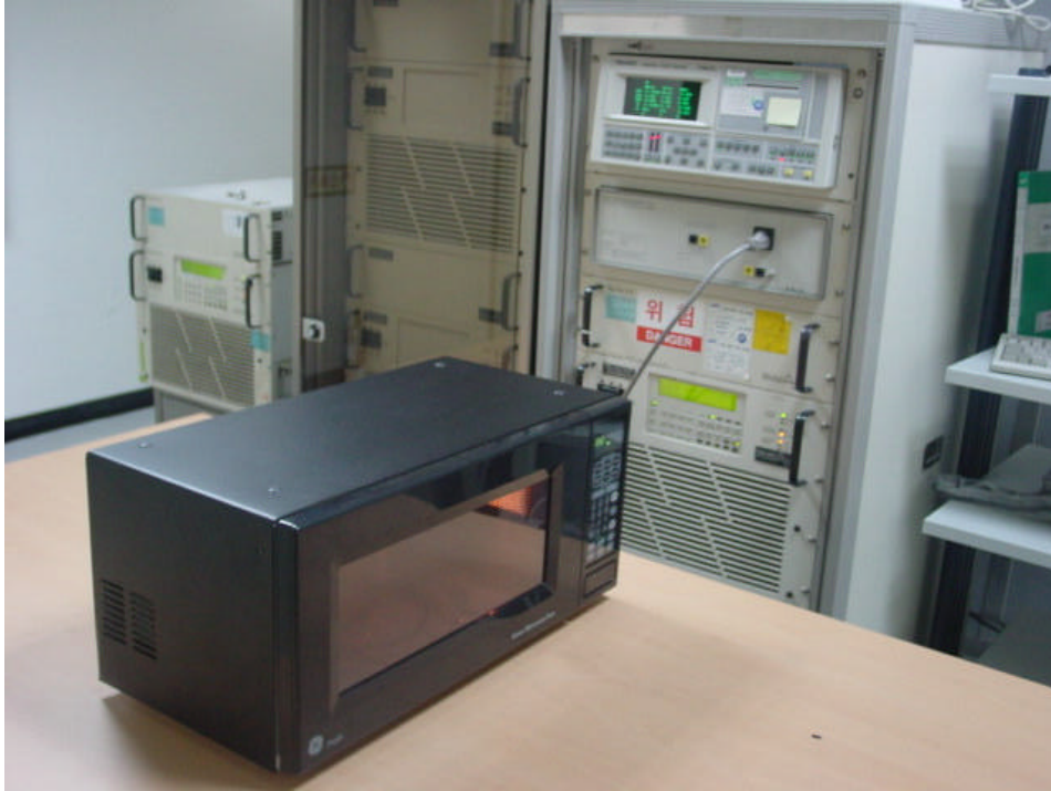
Fig. 2 Test Setup for Operating Frequency Measurements
