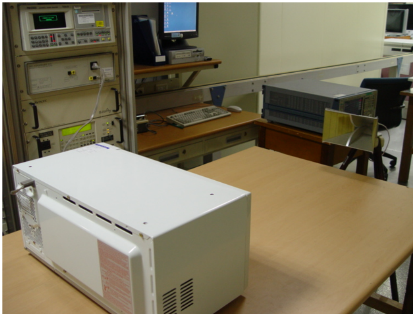
Fig. 2 Test Setup for Input power
