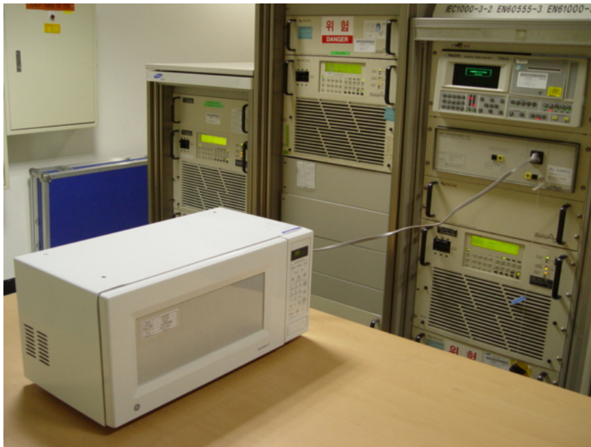
Fig.3 Test Setup for RF output power
