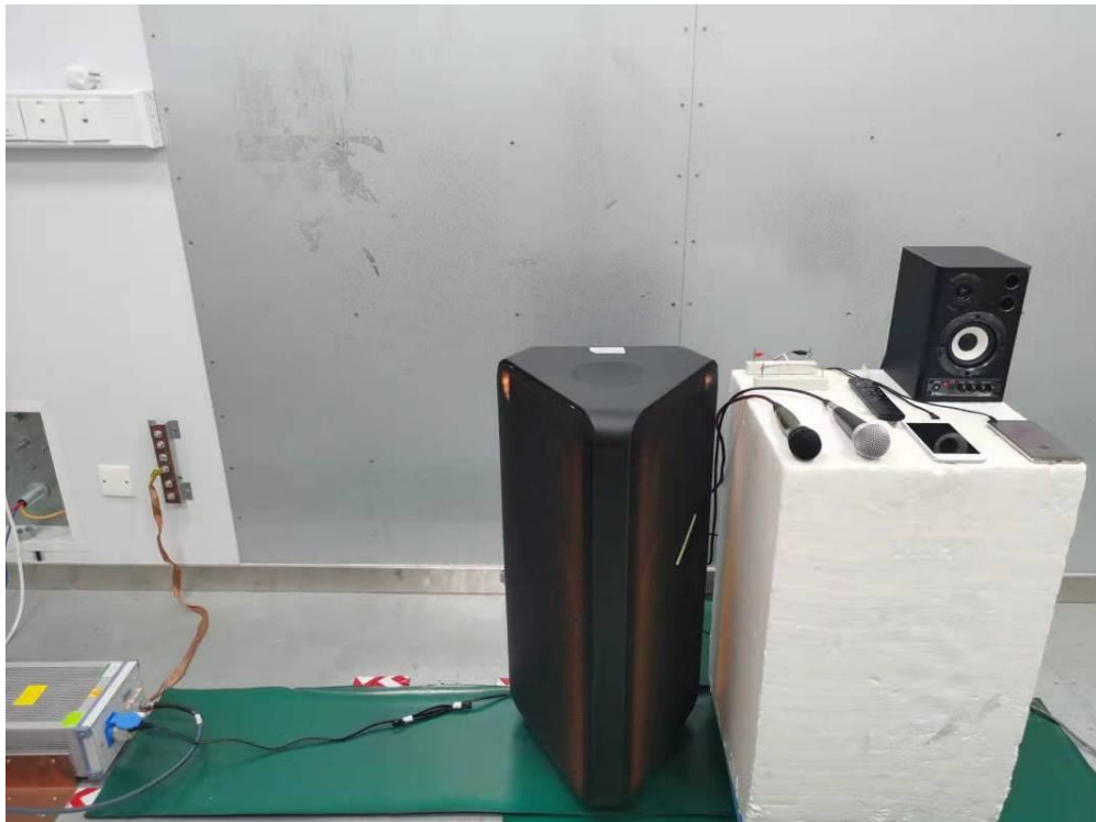
POWERLINE CONDUCTED EMISSIONS MEASUREMENT SETUP
