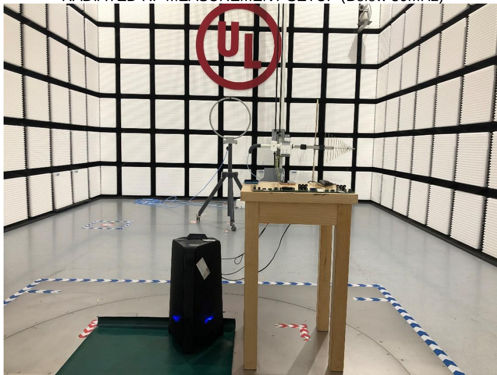
RADIATED RF MEASUREMENT SETUP (Below 30MHz)
