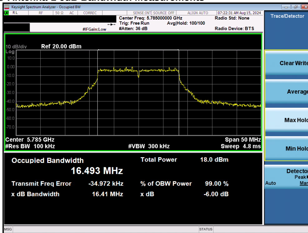
Plot 7-61. 6dB Bandwidth Plot MIMO ANT1 (802.11a (UNII Band 3) – Ch. 157)
