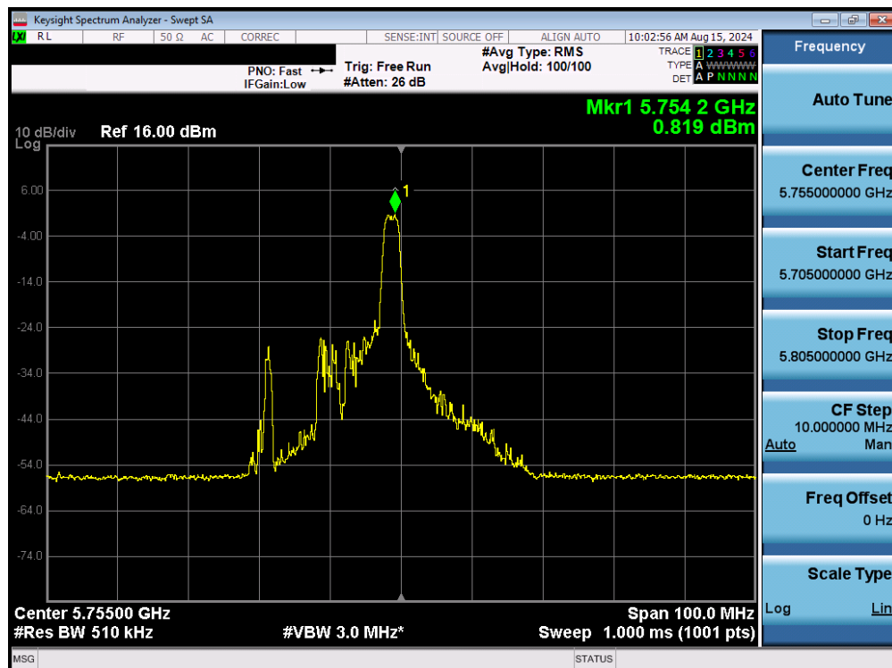
Plot 7-111. Power Spectral Density Plot MIMO ANT1 (40MHz BW 802.11be – 26 Tones (UNII Band 3) – Ch. 151)
