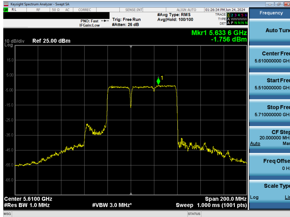
Plot 7-190. Power Spectral Density Plot MIMO ANT2 (80MHz BW 802.11be – 484+242Tones (UNII Band 2C) – Ch. 122)
