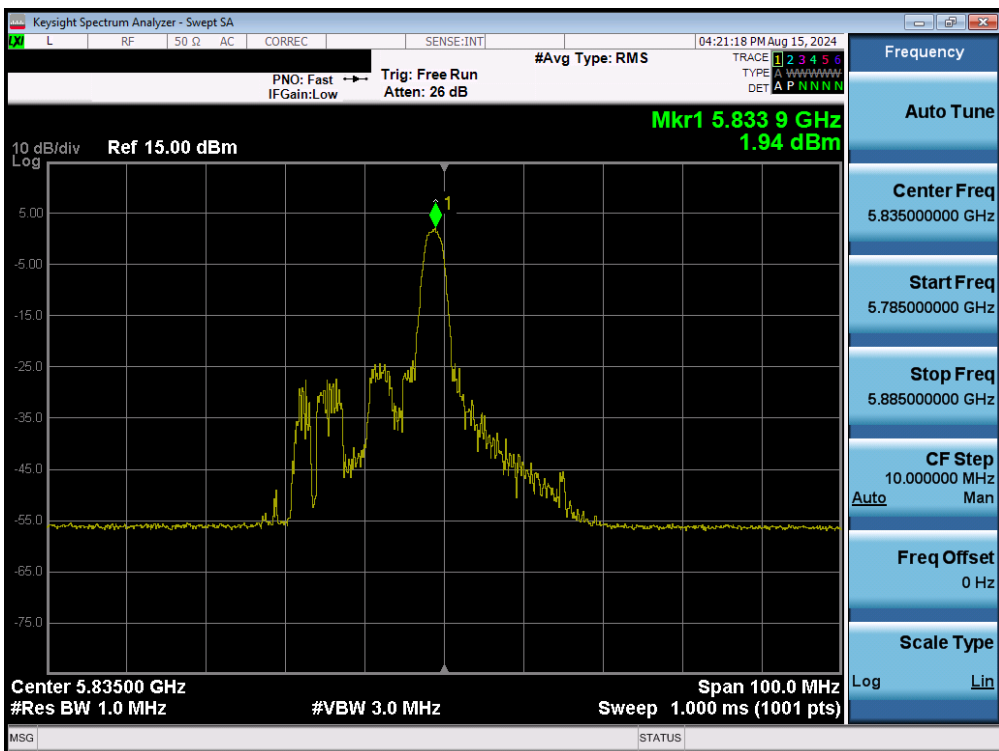
Plot 7-163. Power Spectral Density Plot MIMO ANT2 (40MHz BW 802.11be – 26 Tones (UNII Band 3/4) – Ch. 167)
