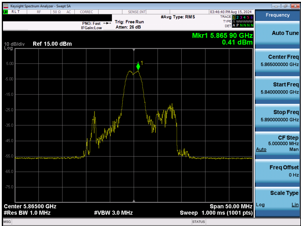
Plot 7-162. Power Spectral Density Plot MIMO ANT2 (20MHz BW 802.11be – 26 Tones (UNII Band 4) – Ch. 173)
