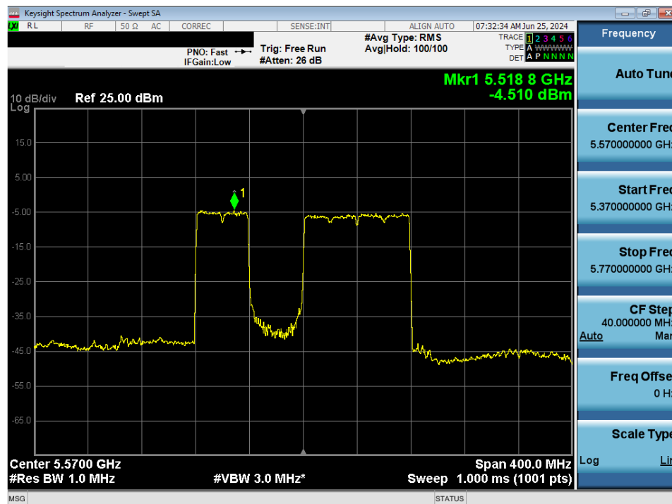
Plot 7-191. Power Spectral Density Plot MIMO ANT2 (160MHz BW 802.11be – 996+484 Tones (UNII Band 2C) – Ch. 114)
