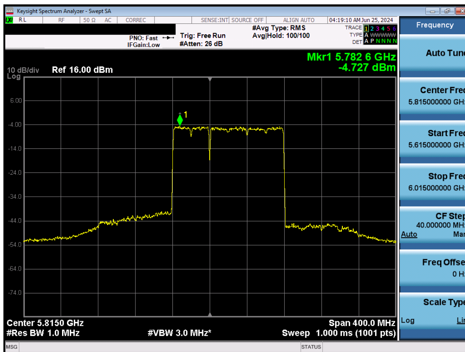
Plot 7-147. Power Spectral Density Plot MIMO ANT1 (160MHz BW 802.11be – 996+484 Tones (UNII Band 3/4) – Ch. 163)
