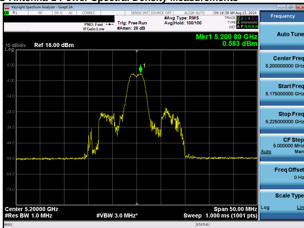
Plot 7-99. Power Spectral Density Plot MIMO ANT1 (20MHz BW 802.11be – 26 Tones (UNII Band 1) – Ch. 40)
