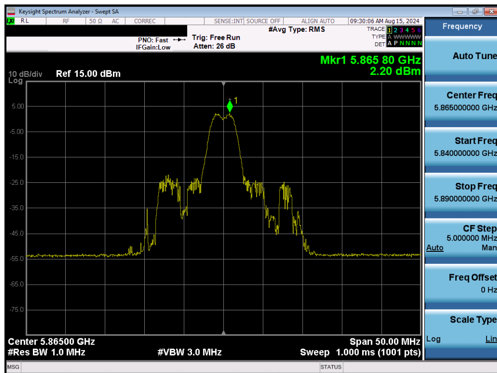
Plot 7-113. Power Spectral Density Plot MIMO ANT1 (20MHz BW 802.11be – 26 Tones (UNII Band 4) – Ch. 173)
