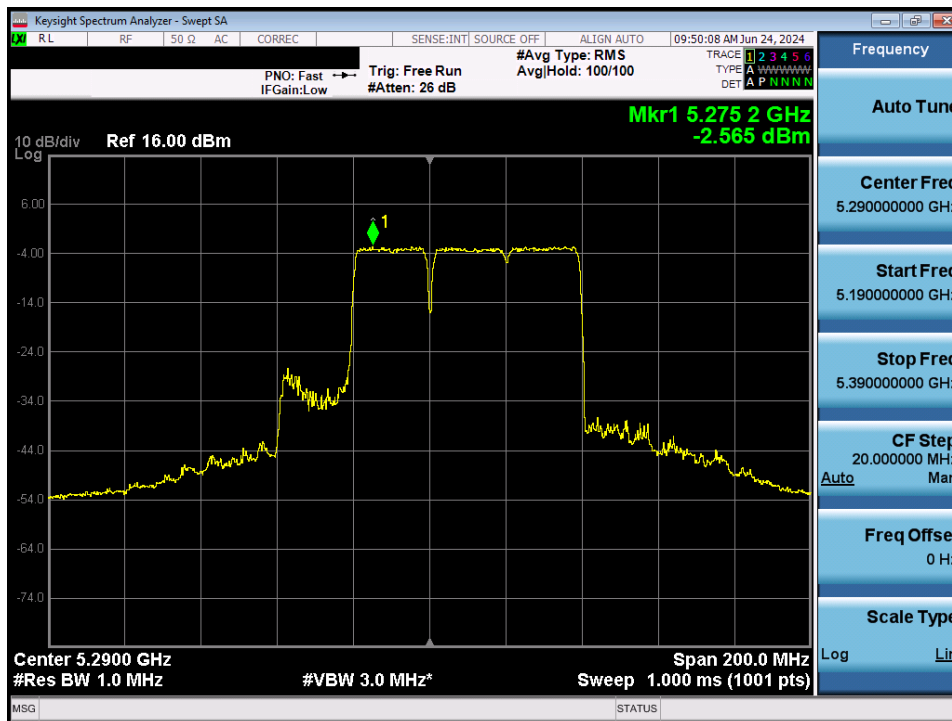
Plot 7-139. Power Spectral Density Plot MIMO ANT1 (80MHz BW 802.11be – 484+242Tones (UNII Band 2A) – Ch. 58)
