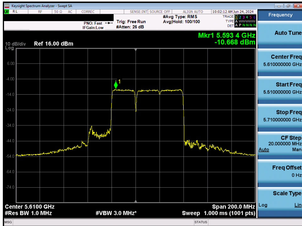
Plot 7-141. Power Spectral Density Plot MIMO ANT1 (80MHz BW 802.11be – 484+242Tones (UNII Band 2C) – Ch. 122)
