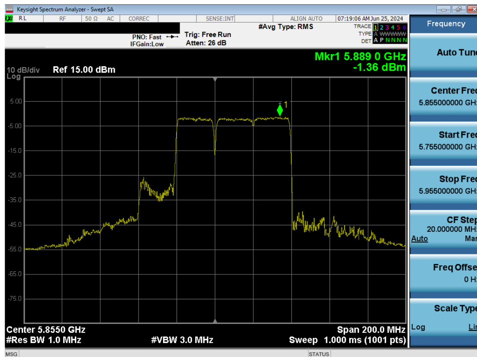
Plot 7-195. Power Spectral Density Plot MIMO ANT2 (80MHz BW 802.11be – 484+242Tones (UNII Band 3/4) – Ch. 171)
