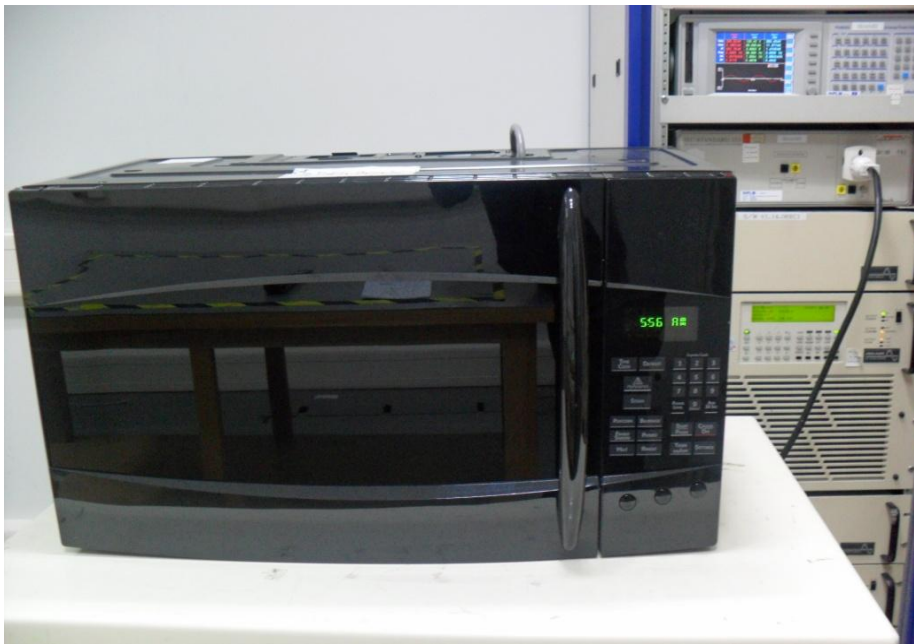
Fig. 2 Test Setup for Input power
