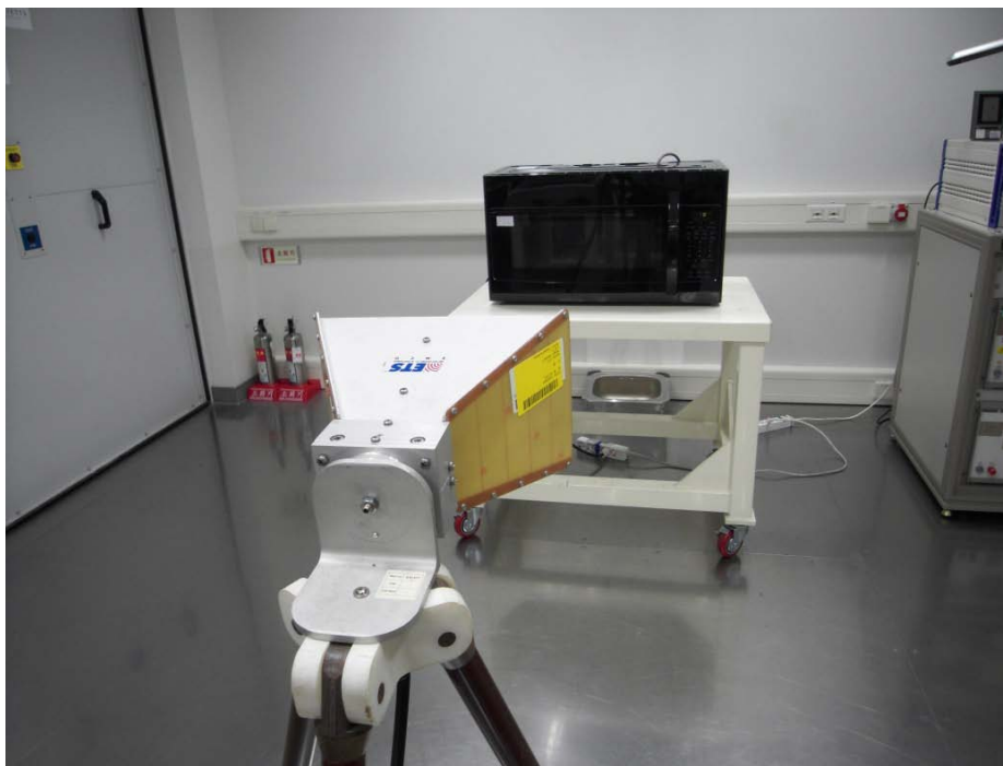
Fig. 4 Operating Frequency Measurements Configuration
