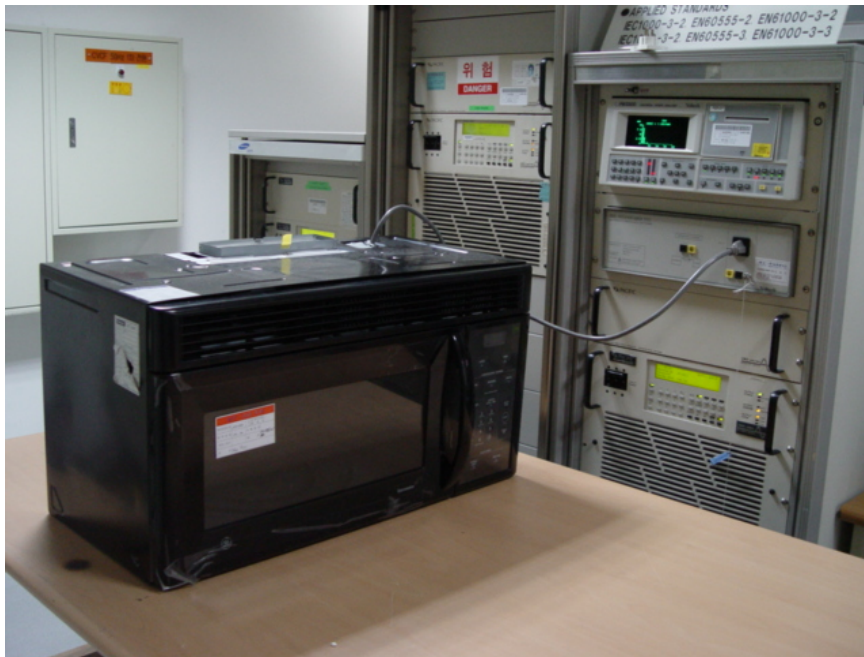
Fig. 2 Test Setup for Input power
