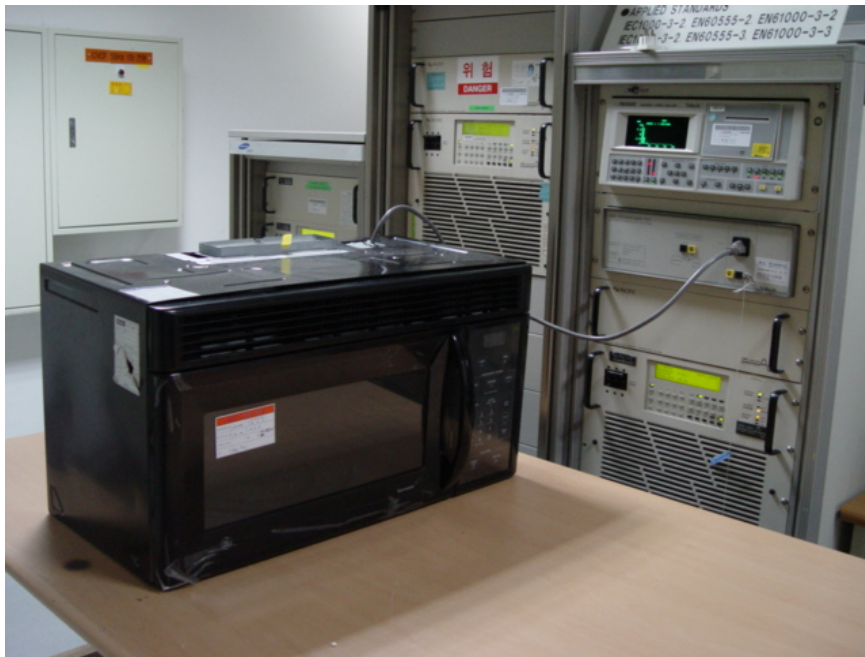
Fig. 2 Test Setup for Input power
