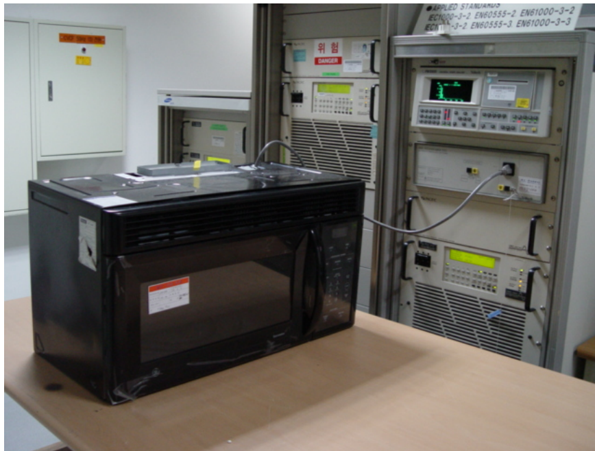
Fig.3 Test Setup for RF output power
