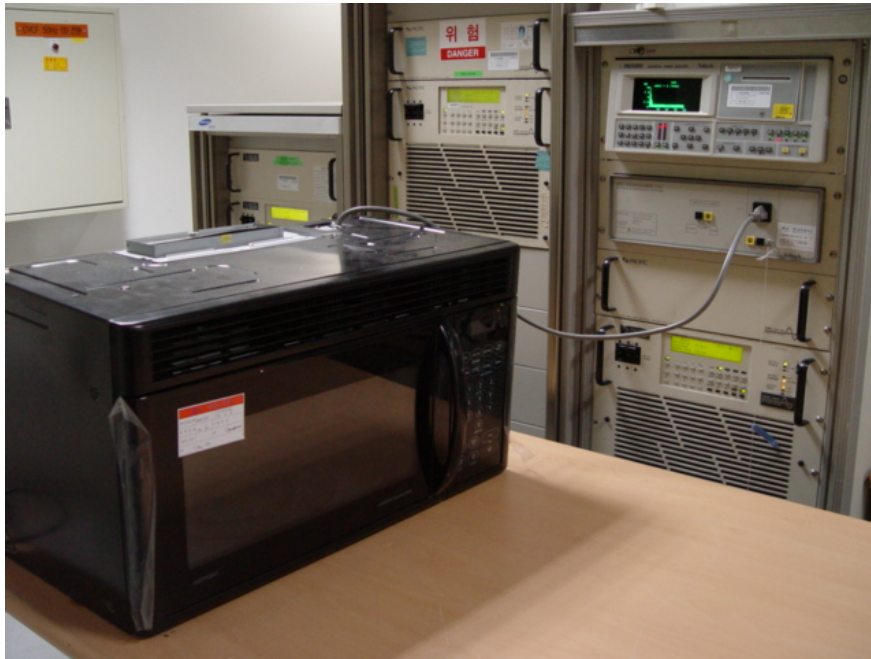
Fig. 2 Test Setup for Input power
