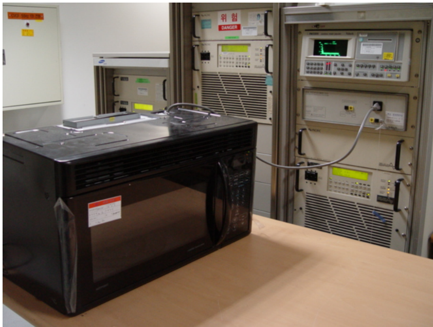
Fig.3 Test Setup for RF output power
