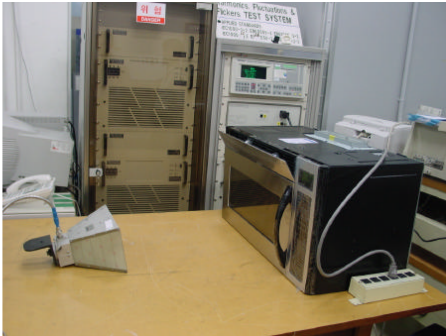
Fig. 2 Test Setup for Input power
