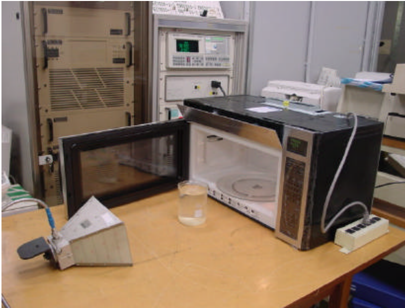
Fig.3 Test Setup for RF output power
