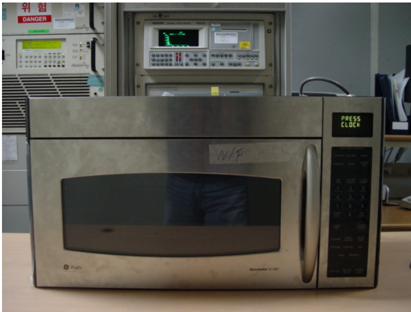
Fig.3 Test Setup for RF output power
