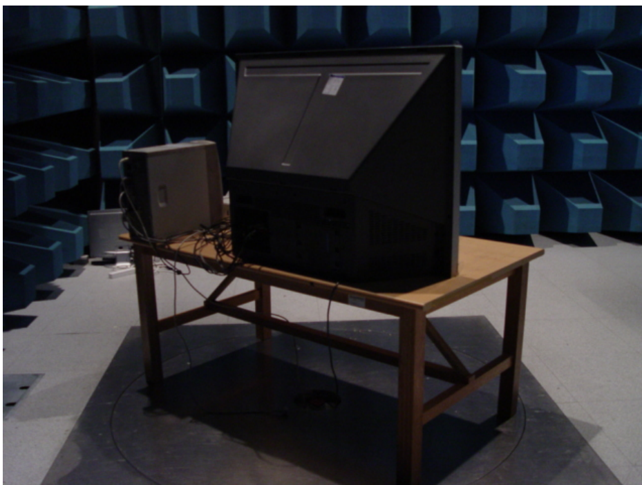
Picture 4. Radiated Emission (Rear)
