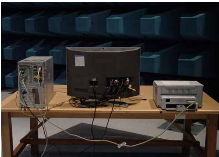
Picture 4. Radiated Emission (Rear)
