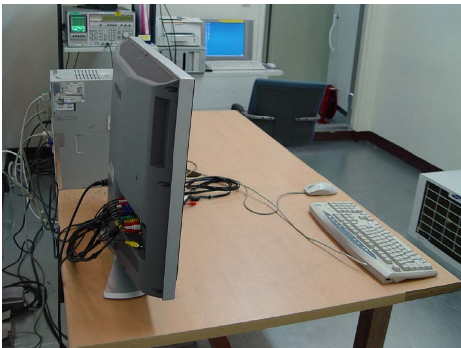
Picture 2. Conducted Emission (Side)
