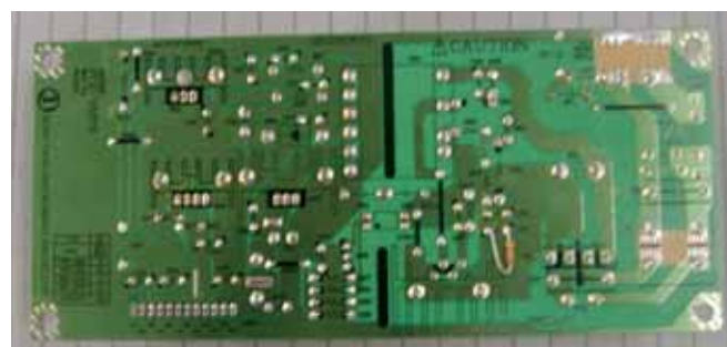
SMPS board bottom view
