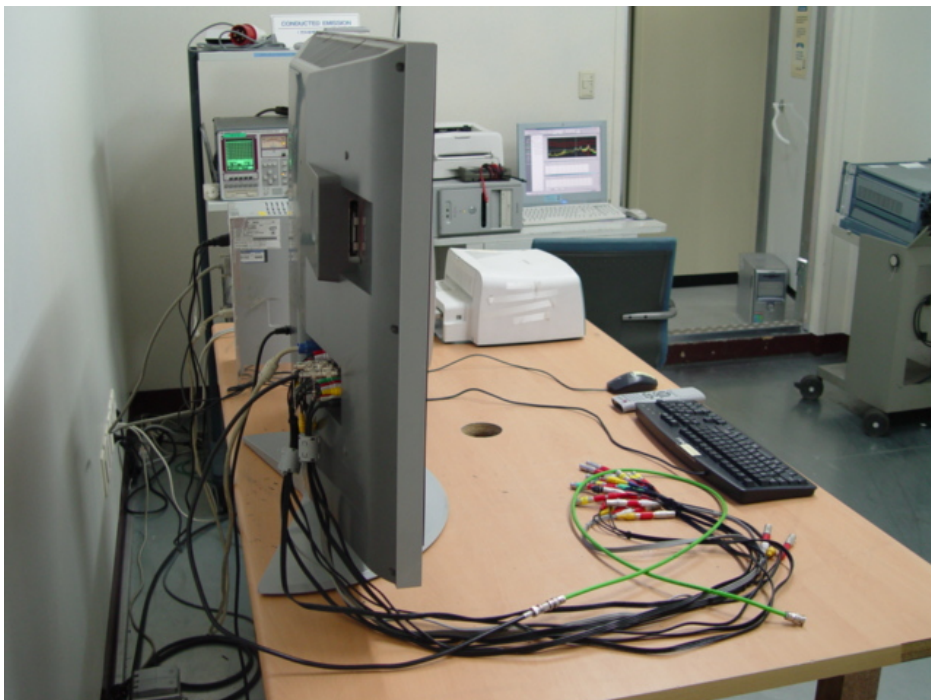
Picture 2. Conducted Emission (Rear)
