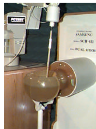
Figure 1. SAR Test Set-up
