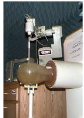
Fig. 1 SAR Test Setup
