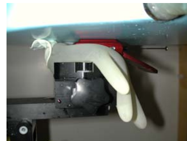
Figure 19. Hand SAR Test Setup
