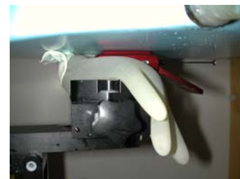
Figure 19. Hand SAR Test Setup
