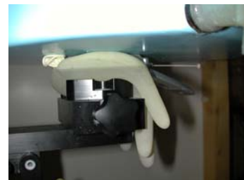
Figure 19. Hand SAR Test Setup
