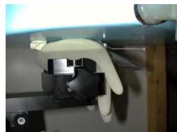
Figure 19. Hand SAR Test Setup
