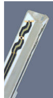
Figure 3.4 Probe Thick-Film Technique
