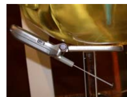
Figure 14.7 Left Head SAR Test Setup -- Left Cheek/ Touch --
