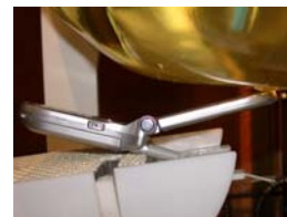
Figure 14.8 Left Head SAR Test Setup -- Left Tilt Position --
