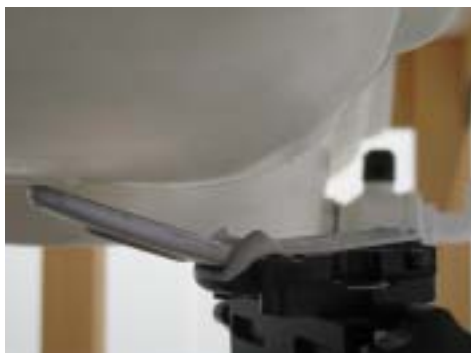
Figure 8.7 Right Head SAR Test Setup -- Ear/Tilt 15° Position--
