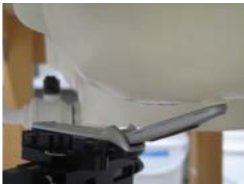
Figure 8.9 Left Head SAR Test Setup -- Ear/Tilt 15° Position--
