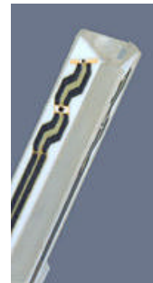
Figure 3.4 Probe Thick-Film Technique
