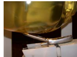
Figure A.6 Right Head SAR Test Setup -- Ear / 15° Tilt Position --
