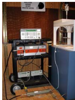
Figure A.0 Dipole Validation Test Setup
