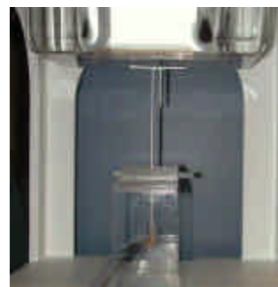
Figure A.0 Dipole Validation Test Setup
