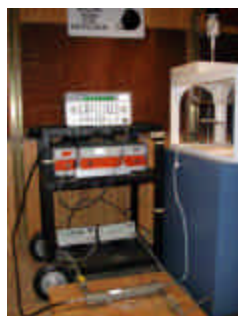
Figure A.0 Dipole Validation Test Setup
