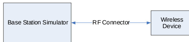
Figure 13-1 Power Measurement Setup
