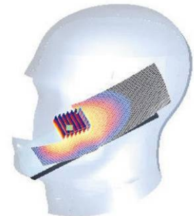
Figure 7-1 Sample SAR Area Scan
