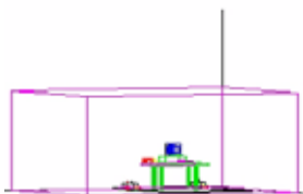
Figure 3-1. Shielded Enclosure Line-Conducted Test Facility
