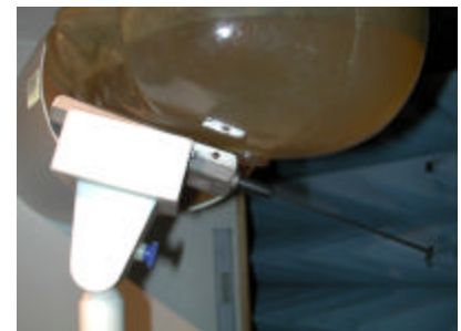
Figure 15. Head SAR Test Setup
