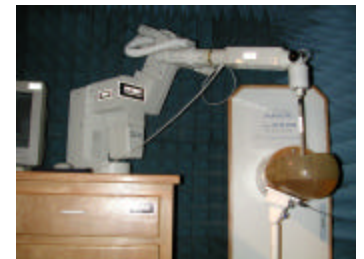
Fig. 1 SAR Test Setup
