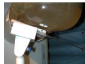
Fig. 14 Head SAR Test Setup
