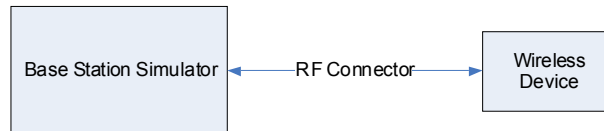
Figure 11-1 Power Measurement Setup
