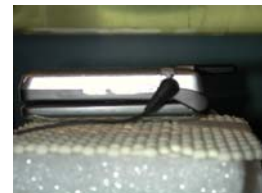
Figure 14.10 Body SAR Test Setup -- w/o Holster --
