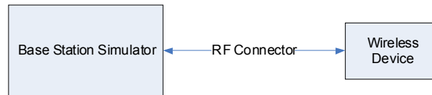
Figure 12-1 Power Measurement Setup
