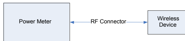
Figure 13-1 Power Measurement Setup
