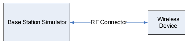
Figure 14-1 Power Measurement Setup
