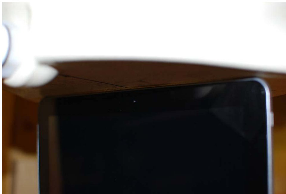
Figure 22-4 SAR Test Setup Photo 4: Top at 0.0 cm
