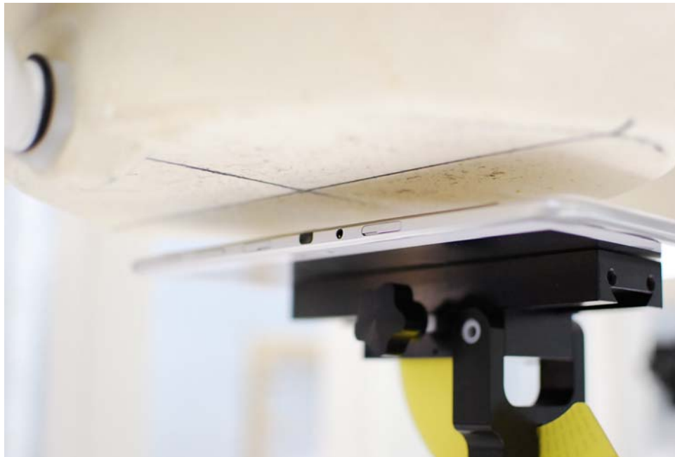
SAR Test Setup Photo 2 – Back Side at 1.4 cm
